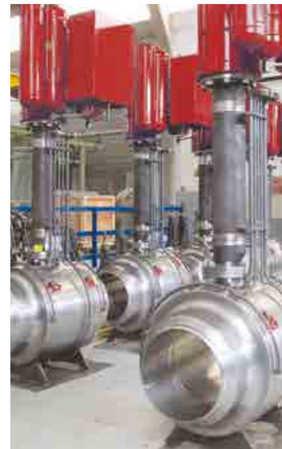
Cryogenic Extended Bonnet With Drip Collar
