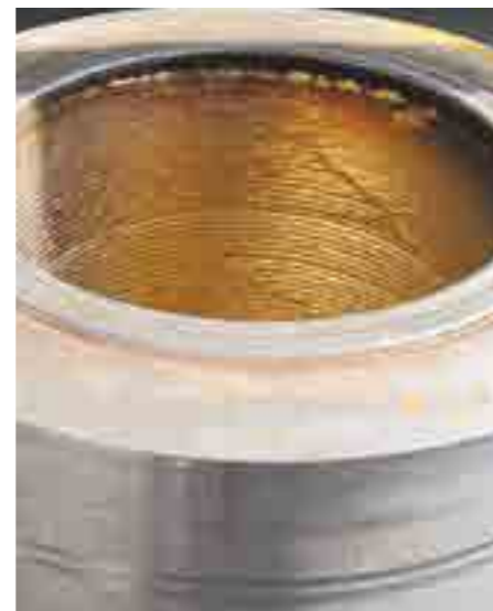
Closure Weld Overlay On All Wetted Parts 3 mm finished thickness.
