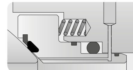
DPE Lubricated Seat - Metal Seated Delta Ring Seal
