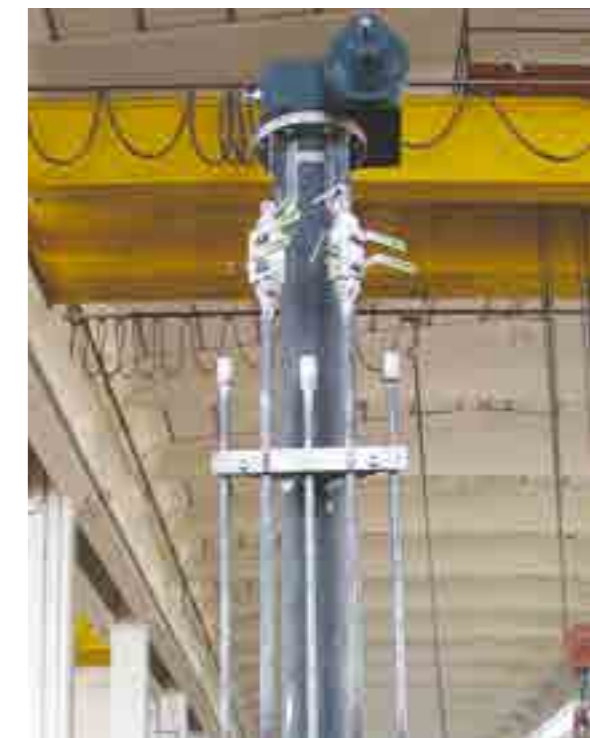
High Temperature Extended Bonnet Live Load Packing
