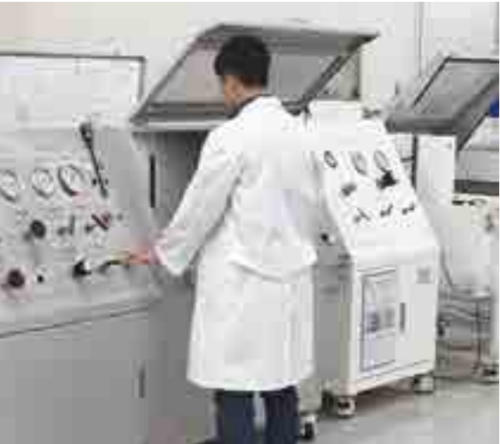
Cryogenic Test - Up to -196°C
