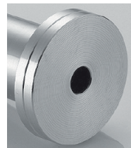
External Groove Concentric Serrated : SR Seal Face Roughness : Ra 6.3 to 12.5 Micrometer
